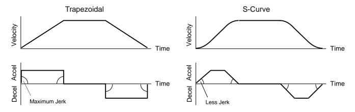
Figure 4-3. S Curve Correction of Moves
